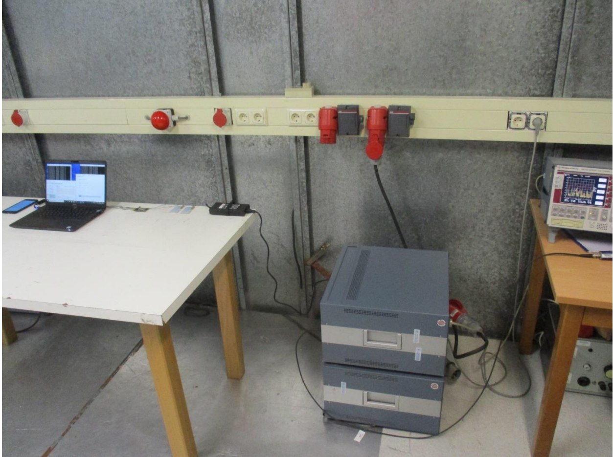
Photo 5: Photograph conducted emissions 0.15-30 MHz
