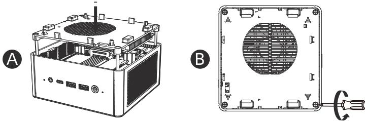
Insert the cable into the connectors and tighten the four screws on the cover.
