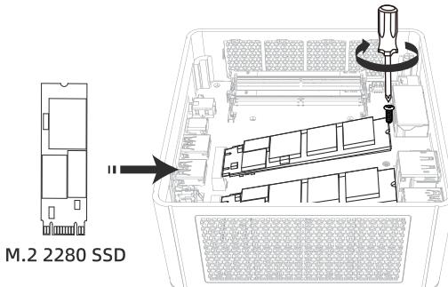
Install the SSD into its slot by inserting it slantly and fix it with screws.
