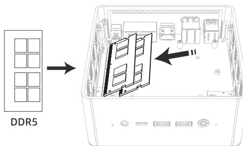
Insert the memory into the memory slot according to the diagram.
