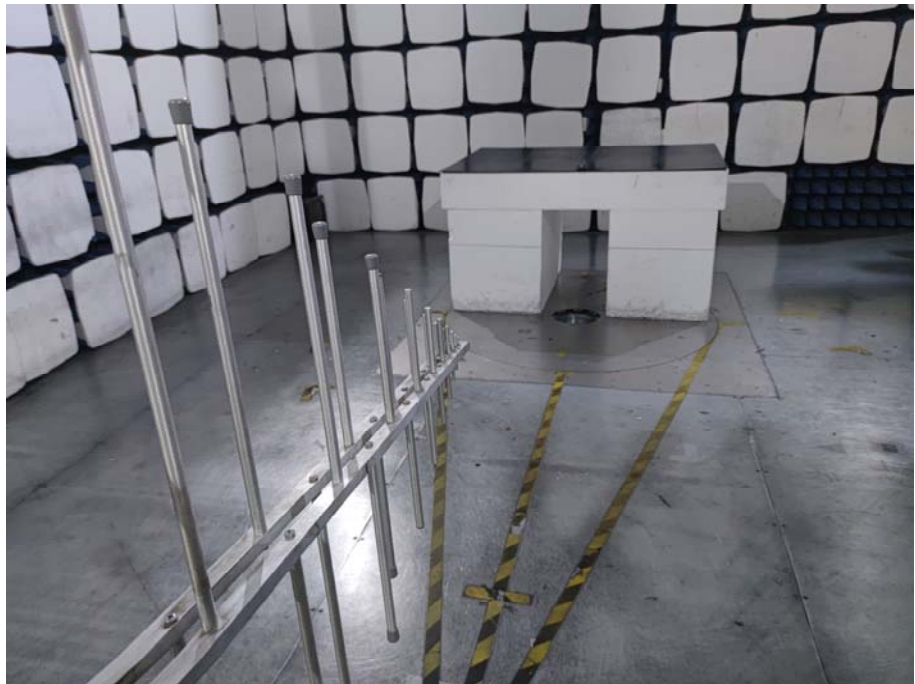
Radiation Emission Test Setup (30MHz to 1GHz)
