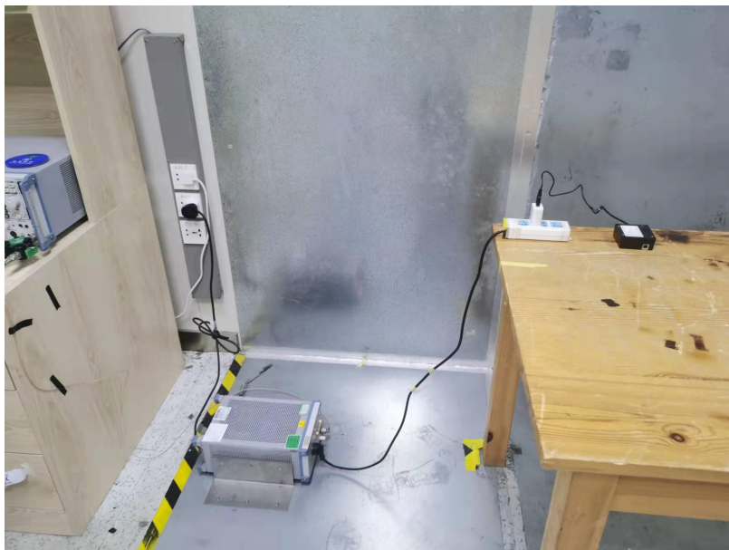
Power Line Conducted Emission Test Frequency From 0.15MHz-30MHz
