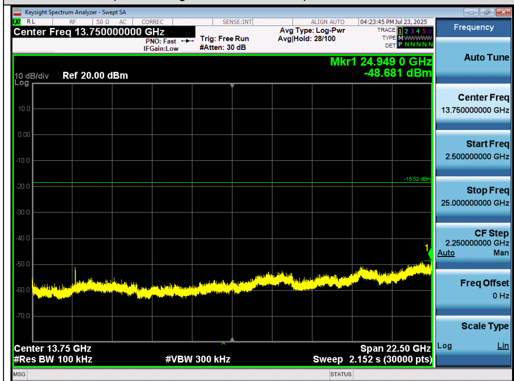
Test_Graph_802.11g_ANT1_2462_6Mbps_Higher Band Emissions
