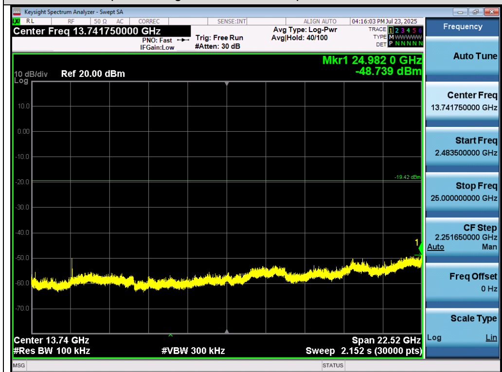
Test_Graph_802.11g_ANT1_2412_6Mbps_Higher Band Emissions
