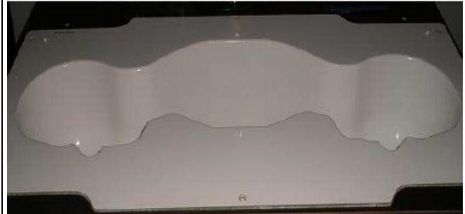
The bottom plate contains three pair of bolts for locking the device holder. The device holder positions are adjusted to the standard measurement positions in the three sections. A white cover is provided to tap the phantom during off-periods to prevent water evaporation and changes in the liquid parameters. On the phantom top, three reference markers are provided to identify the phantom position with respect to the robot.
