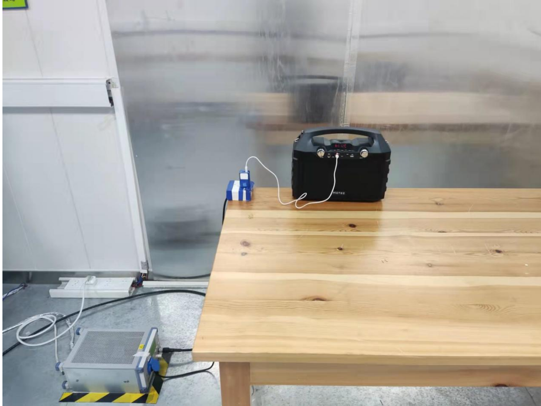
Conducted emission test setup
