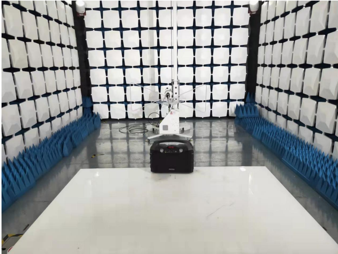
Blow 1GHz for radiated emission test setup
