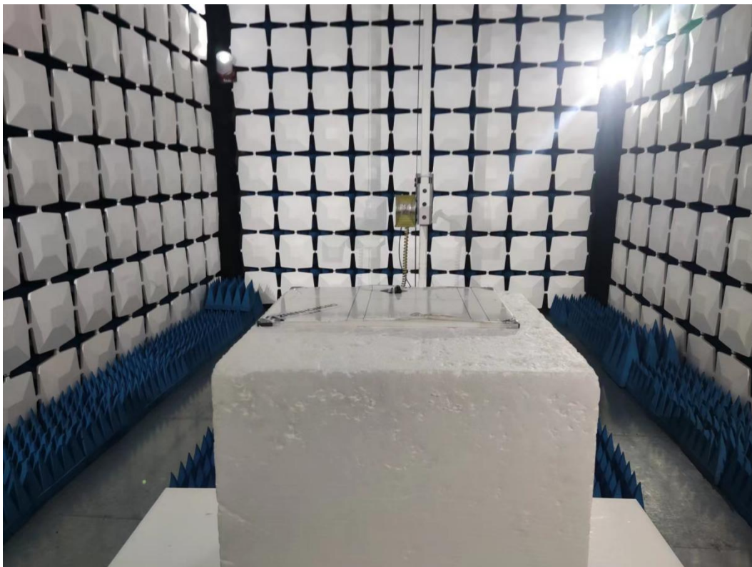
Above 1GHz for radiated emission test setup
