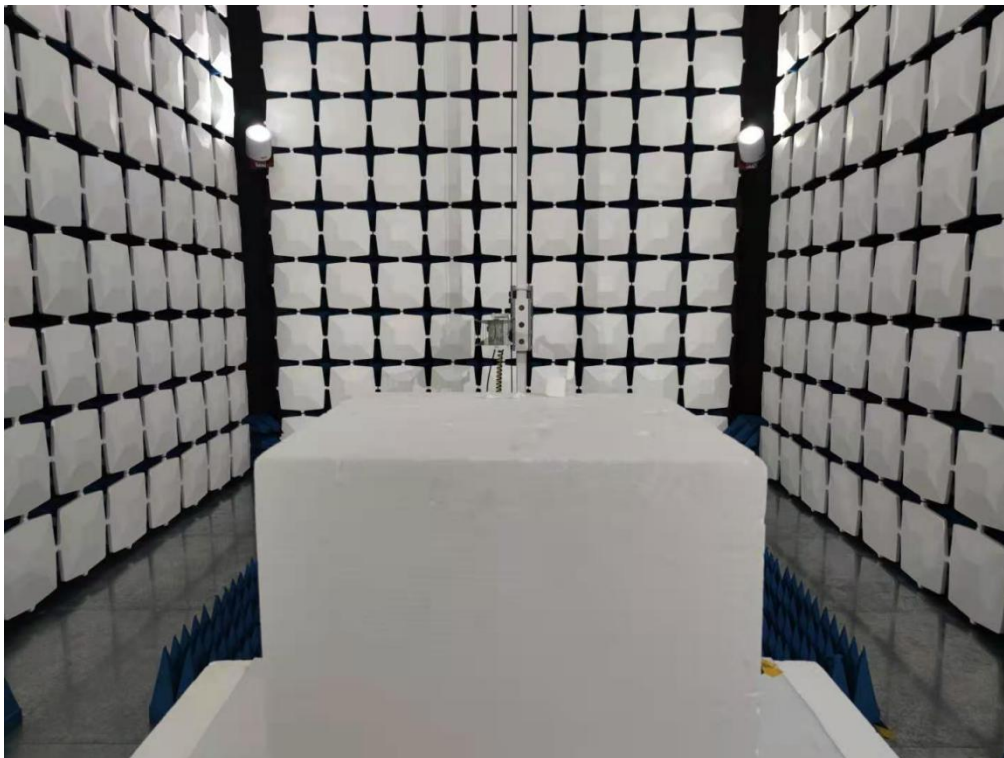
Above 1GHz for radiated emission test setup
