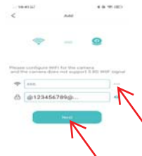
③Click "..." to connect to the local 2.4G WIFI band, enter the password, and then go to the next step
