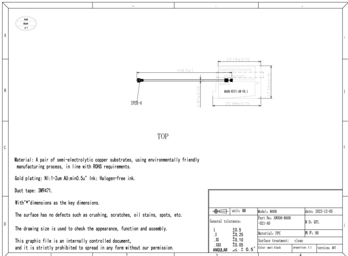
(Working frequency band of 2.4G/5GWIFI antenna) : 2400~2500
