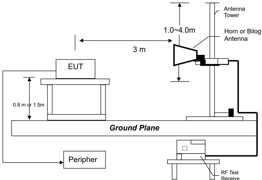
Radiated emission measurements were performed from 9KHz to tenth harmonic or 40GHz.
