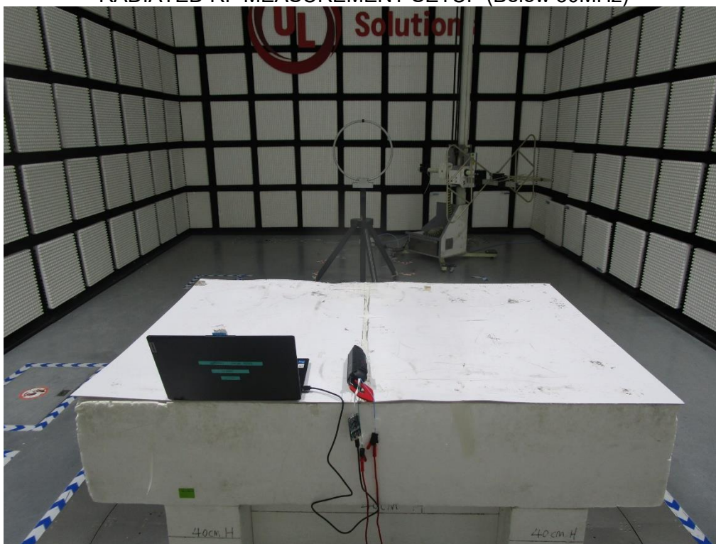
RADIATED RF MEASUREMENT SETUP (Below 30MHz)
