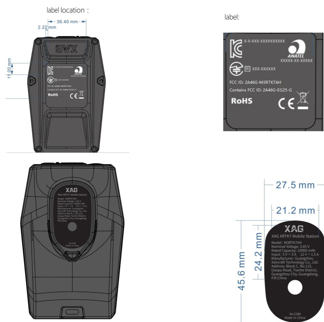
The label is attached to the top of the device with a permanent adhesive.
