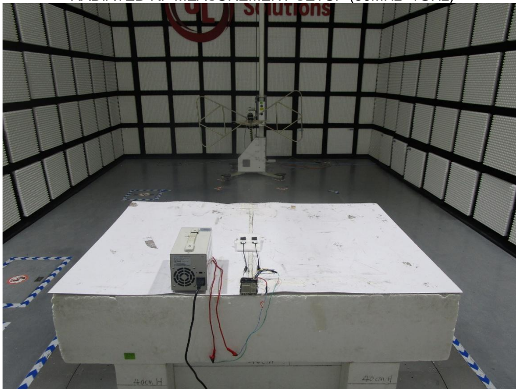
RADIATED RF MEASUREMENT SETUP (30MHz~1GHz)
