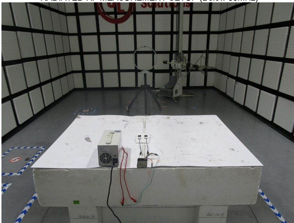
RADIATED RF MEASUREMENT SETUP (Below 30MHz)
