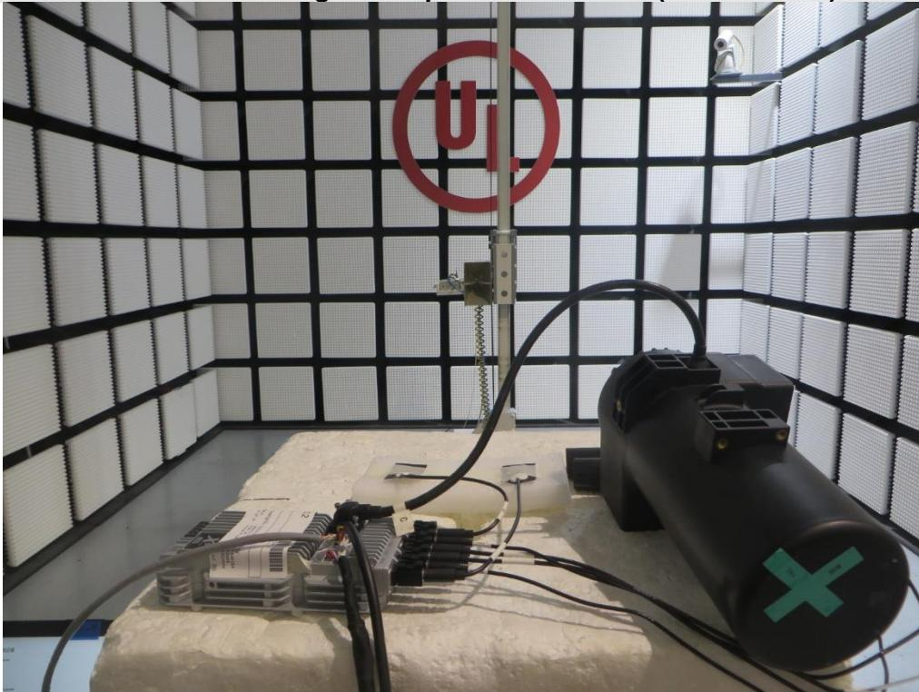
**RADIATED RF MEASUREMENT SETUP (30MHz~1GHz)**
