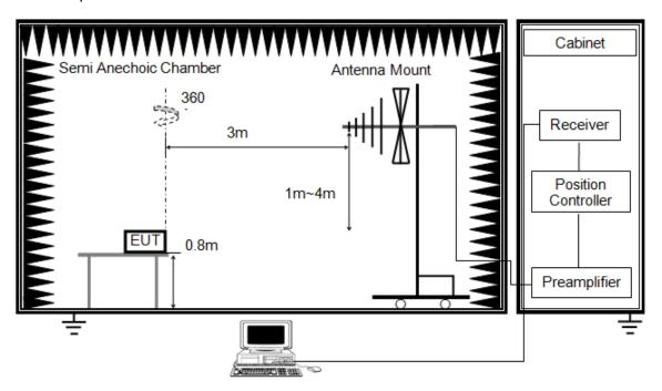
Test Setup for Above 1 GHz
