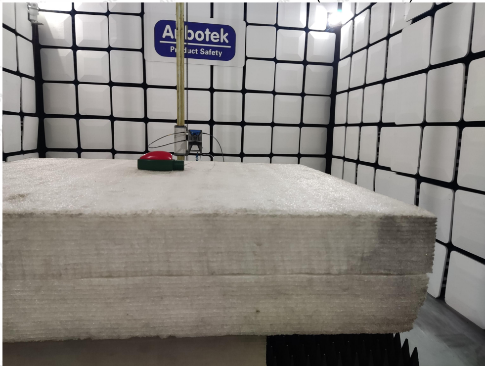
Photo of Radiation Emission Test (above 1GHz)
