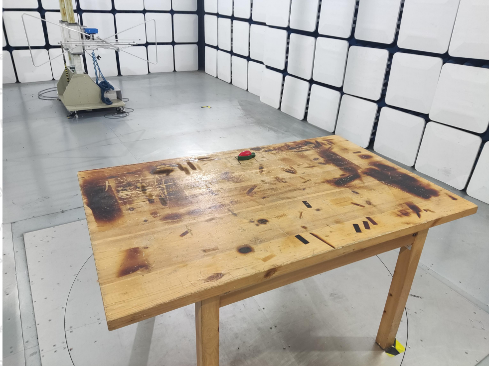
Photo of Radiation Emission Test (below 1GHz)
