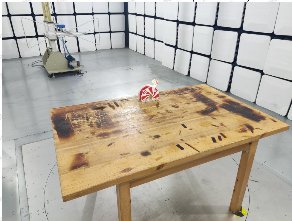
Photo of Radiation Emission Test (below 1GHz)
