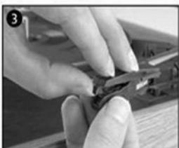
separate the cartridge from the socket lightly.
