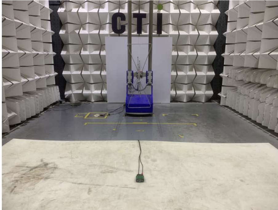
Radiated spurious emission Test Setup-1(Below 1GHz)
