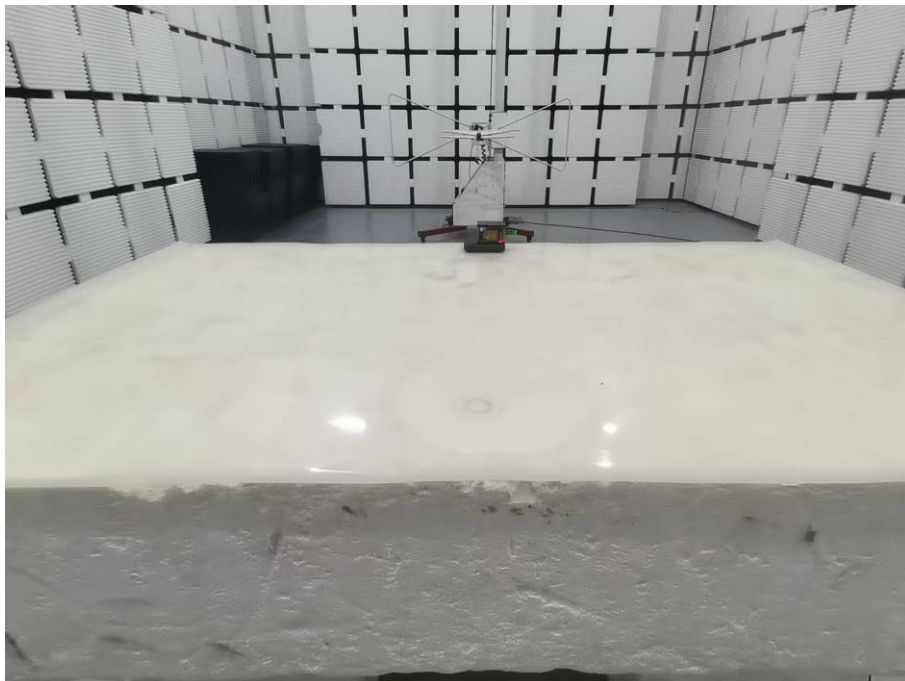
Photograph 2: Set-up photo for Radiated Emission, 30MHz - 1GHz
