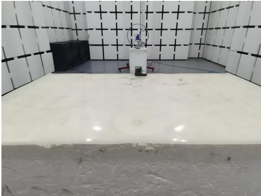
Photograph 1: Set-up photo for Radiated Emission, 9KHz - 30MHz
