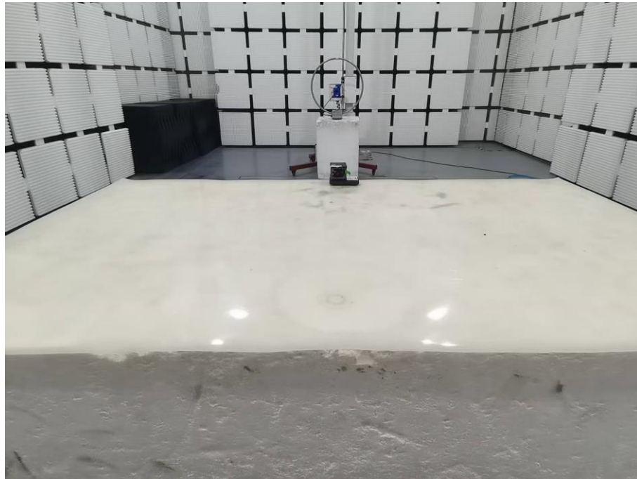
Photograph 1: Set-up photo for Radiated Emission, 9KHz - 30MHz
