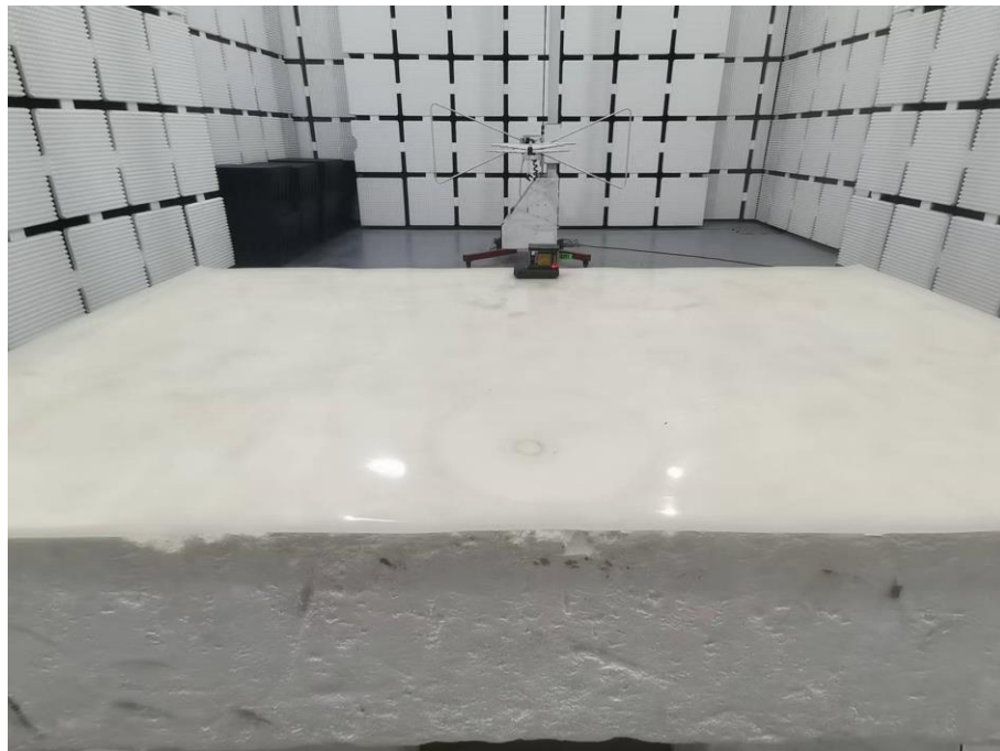
Photograph 2: Set-up photo for Radiated Emission, 30MHz - 1GHz
