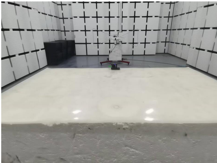
Photograph 2: Set-up photo for Radiated Emission, 30MHz - 1GHz
