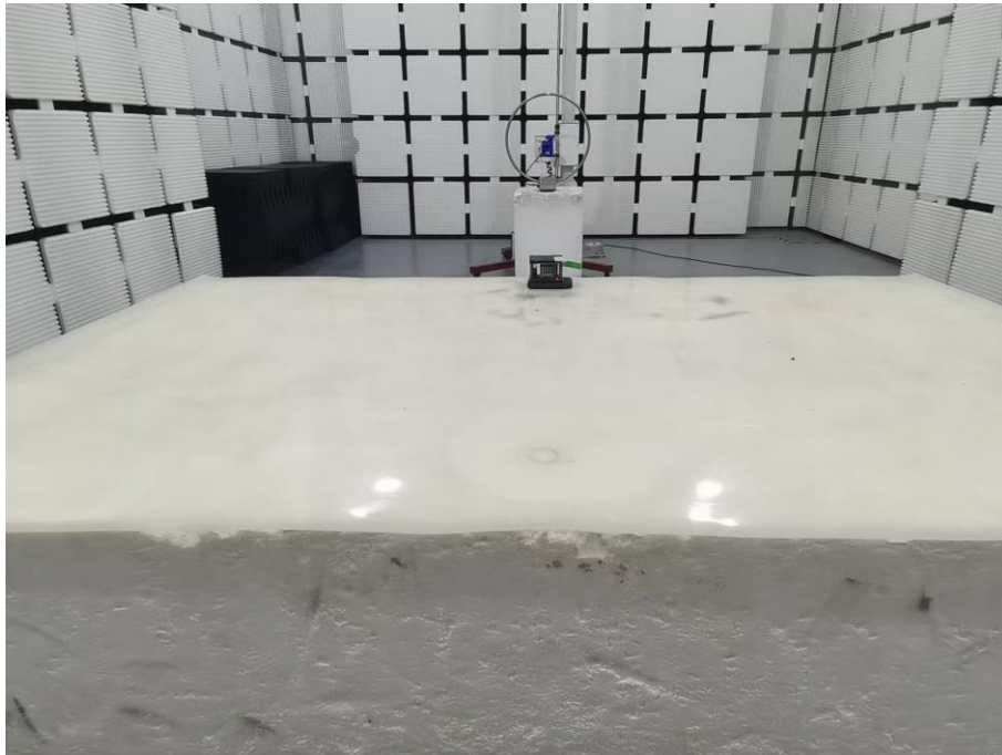
Photograph 1: Set-up photo for Radiated Emission, 9KHz - 30MHz
