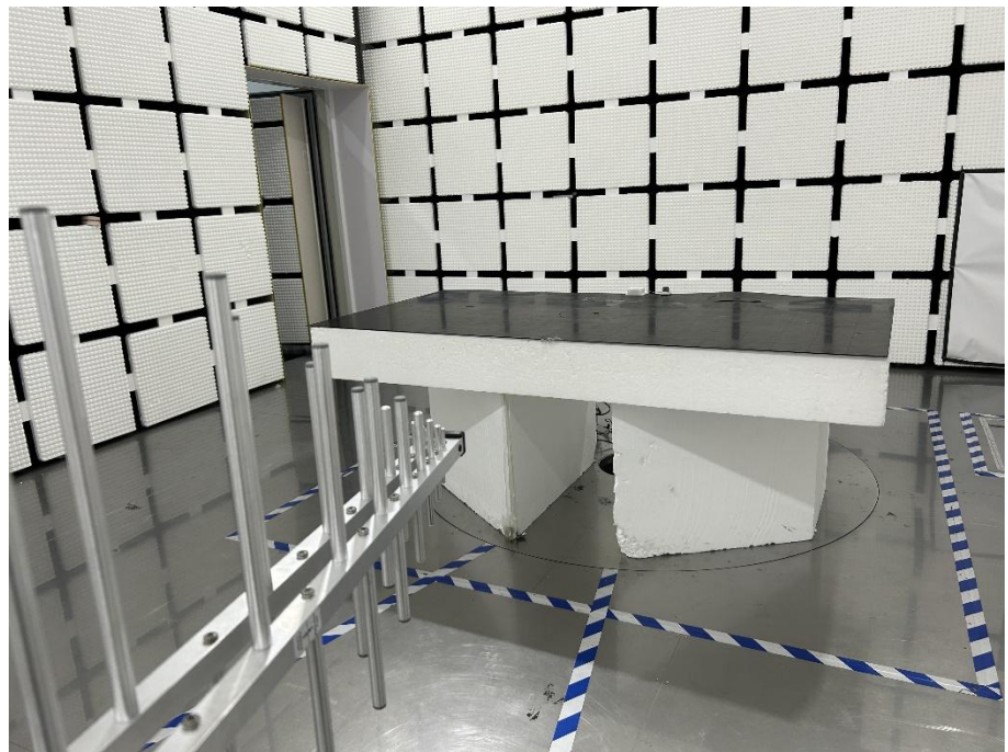
Radiation Emission Test Setup (30MHz to 1GHz)
