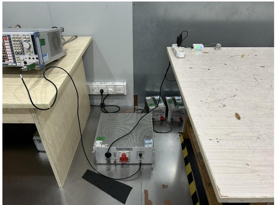
Conducted Emission Test Setup
