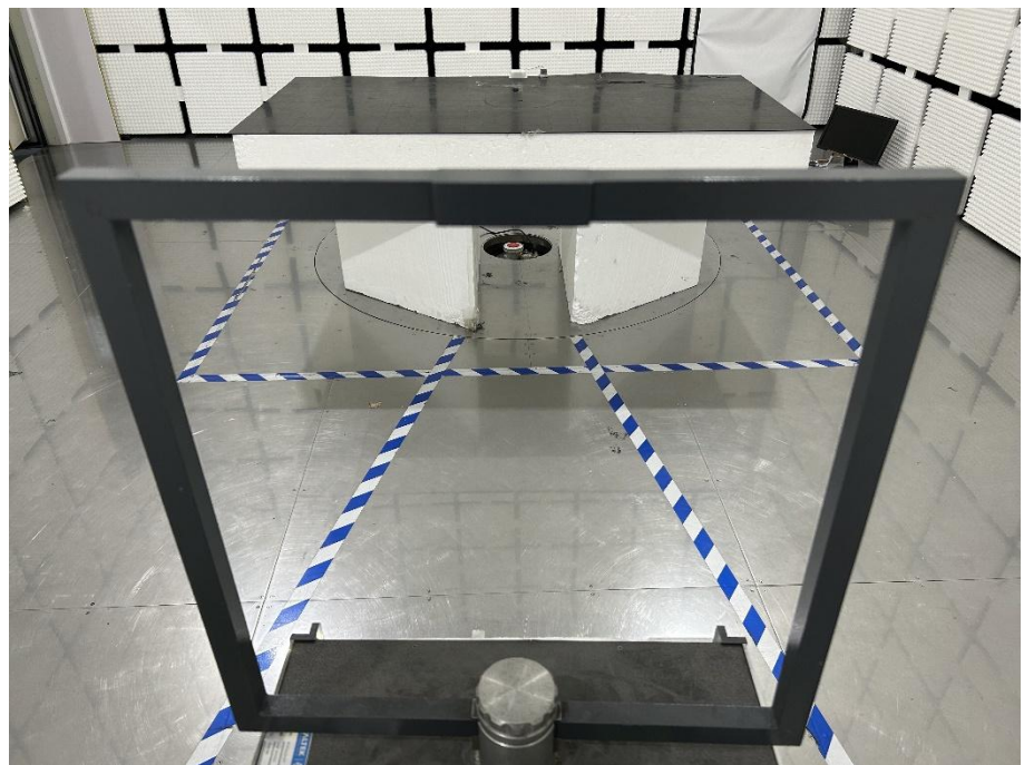
Radiation Emission Test Setup (Below 30MHz)
