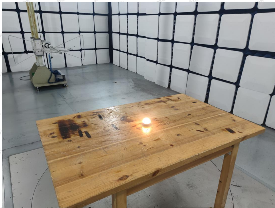
Photo of Radiation Emission Test
