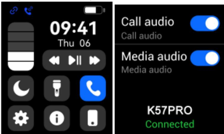
Step4: Check watch menu “about” MAC address last four number like “6326” , then go mobile phone “setting-bluetooth” to search the same bluetooth name with last 4 numbers “6326” to finish BT connection as below operation.
