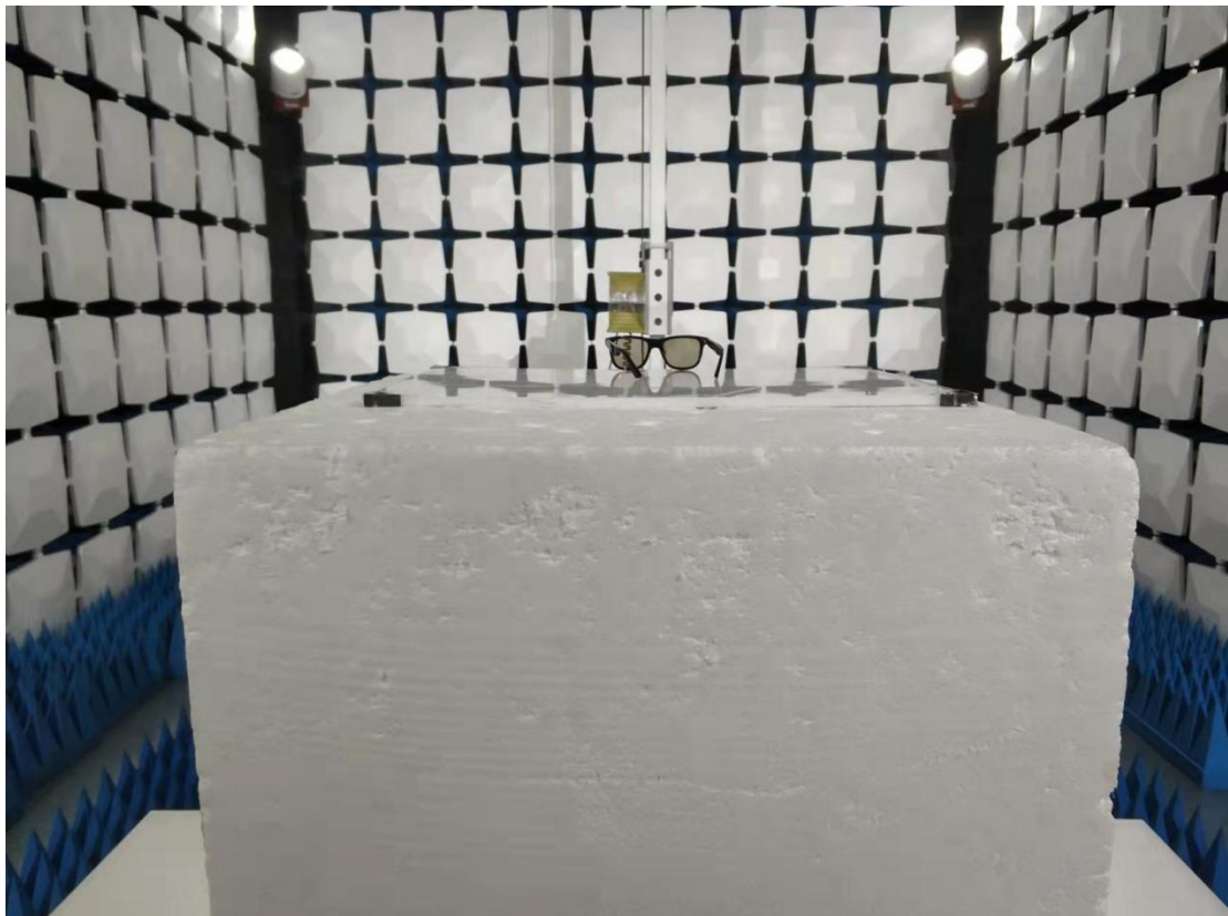
Above 1GHz for radiated emission test setup
