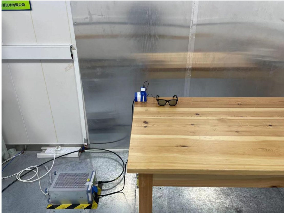
Conducted emission test setup
