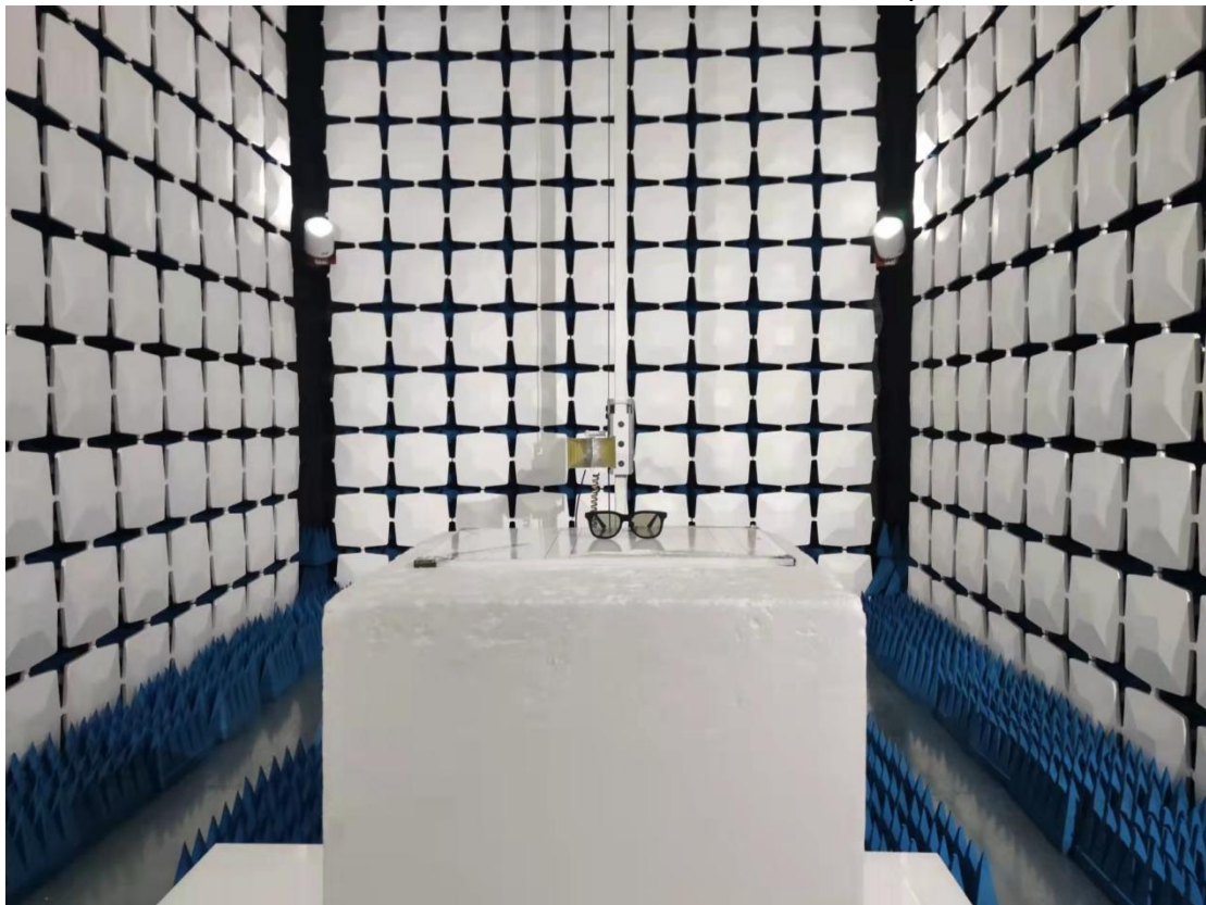
Above 1GHz for radiated emission test setup
