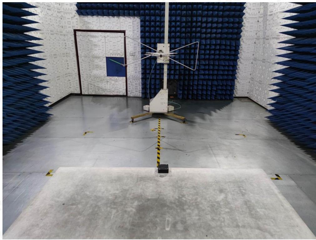
BT RADIATED EMISSION TEST SETUP ABOVE 1GHz
