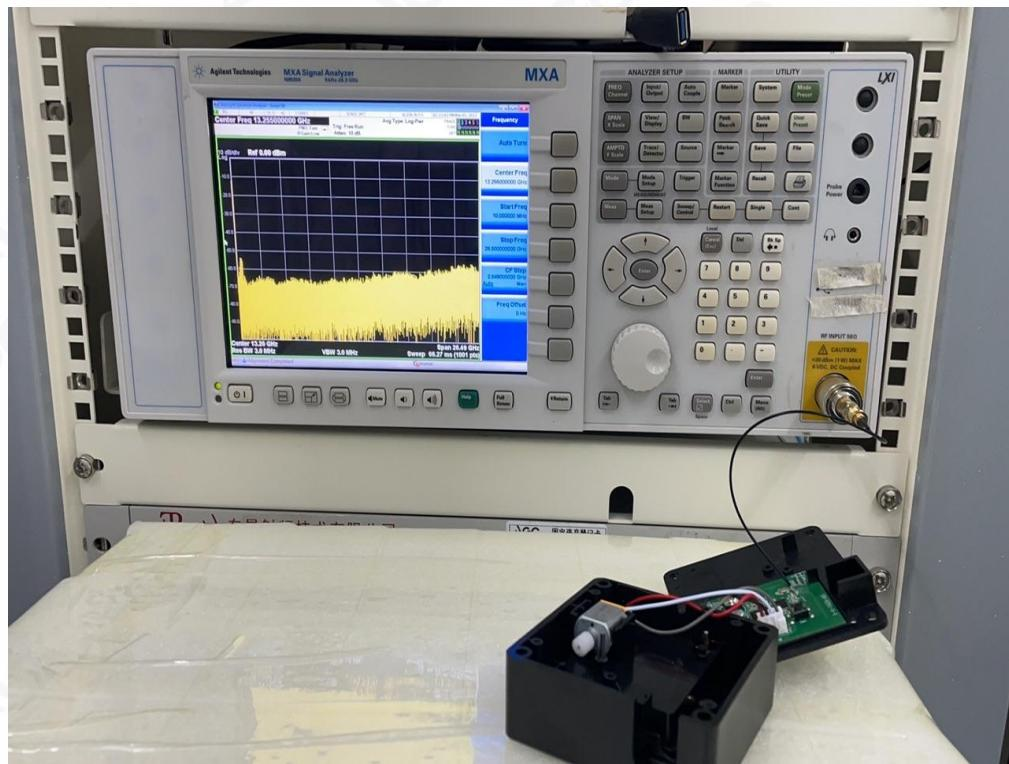
RFID RADIATED EMISSION TEST SETUP BELOW 30MHz
