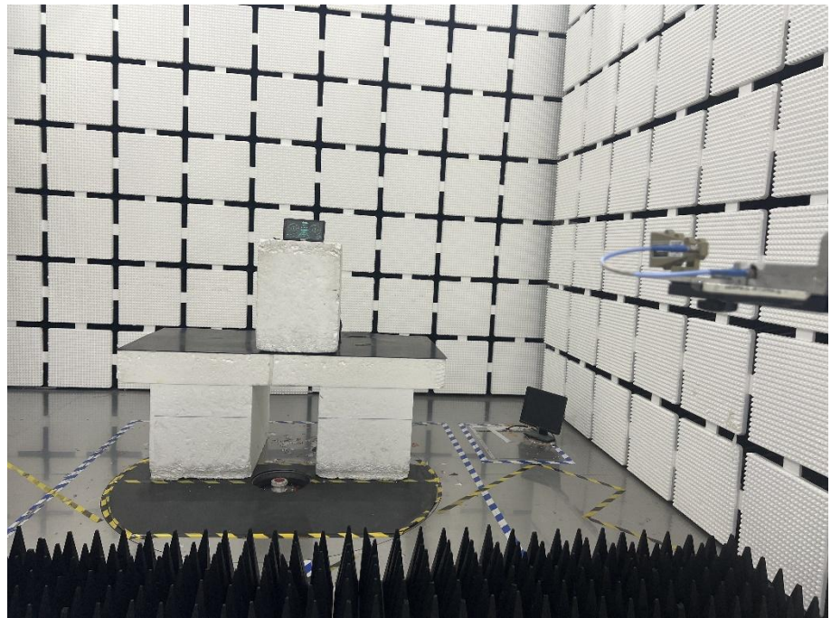
Radiation Emission Test Setup (Above 18GHz)
