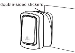
Tip: Please avoid installing on metal objects (iron gates, iron windows, etc.) to avoid affecting the launch distance. Please try it before fixed transmitter.
