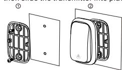
Tip: Please avoid installing on metal objects (iron gates, iron windows, etc.) to avoid affecting the launch distance. Please try it before fixed transmitter.
