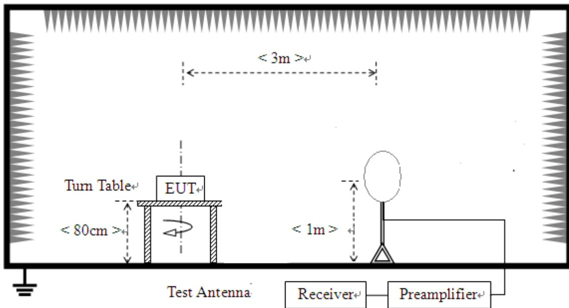
For radiated emissions from 30MHz to 1GHz
