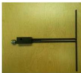
Figure 1 – MVG COMOSAR Validation Dipole
