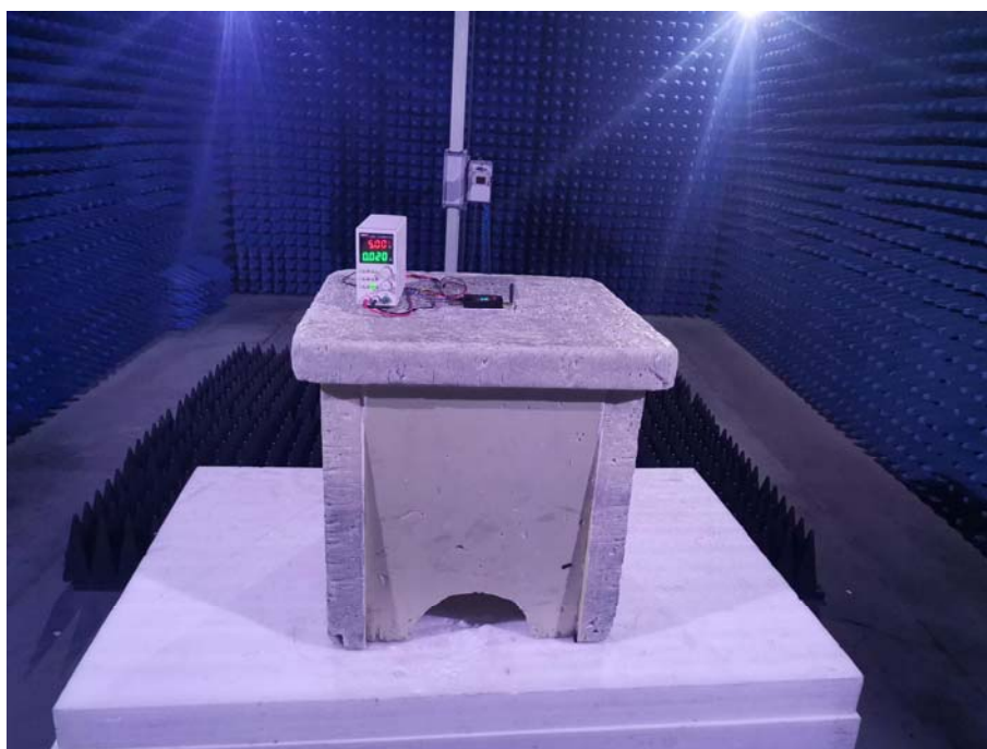
Photo of Radiated Emission Measurement 18-25GHz
