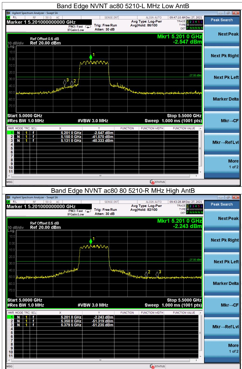
Note: A(B) Represent the value of antenna A and B, The worst data is Antenna B, only shown Antenna B.
