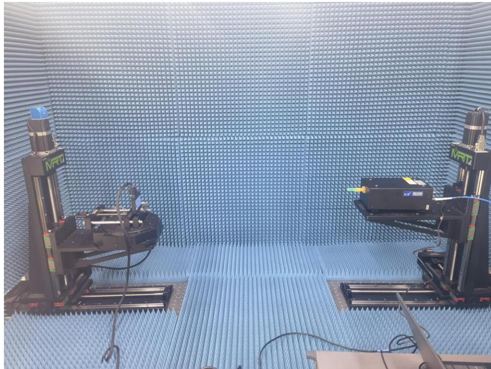
Description: RF Radiated Test Setup
