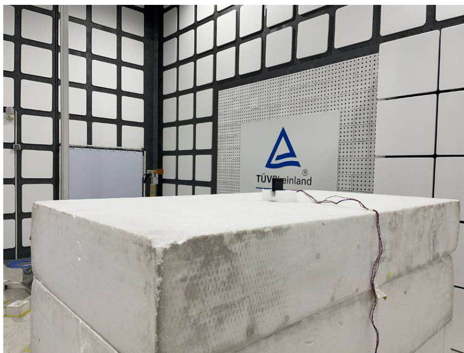
Photograph 6: Set-up photo for Radiated Spurious Emission, Above 75GHz
