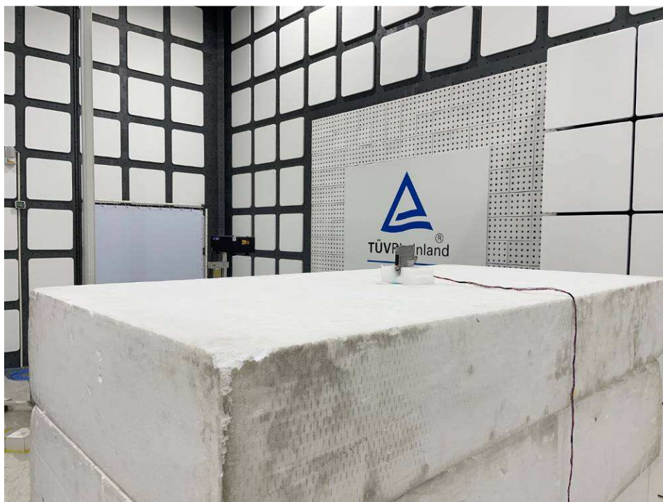
Photograph 6: Set-up photo for Radiated Spurious Emission, Above 75GHz
