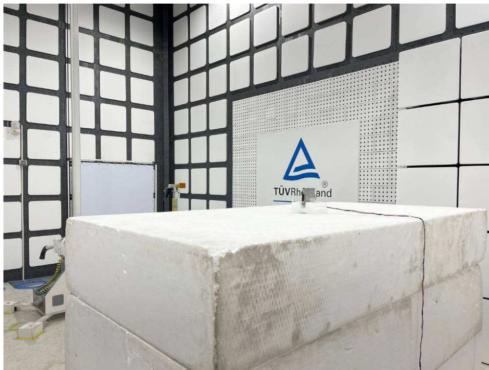
Photograph 6: Set-up photo for Radiated Spurious Emission, Above 75GHz
