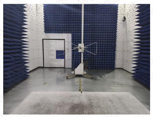
RADIATED EMISSION TEST SETUP ABOVE 1GHz
