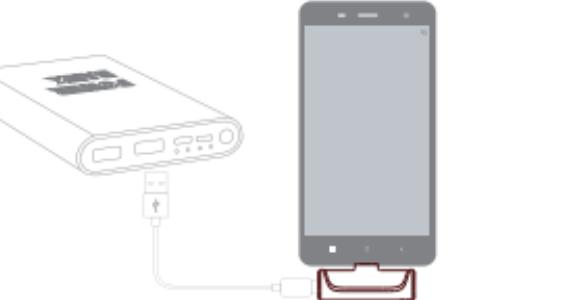
When the microphone is low battery, the indicator of the microphone flashes red light. Charge the microphone with the type-c cable.
