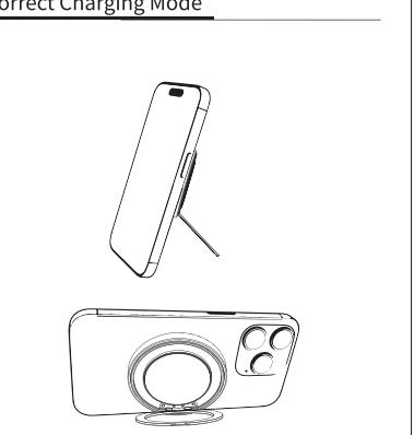
Magnetic wireless charging phones could be charged when the charger stand folded, the phone will attach to the pad well automatically, which could adjust the view angle with your preference. Note: This product supports wireless charging to the wireless charging devices without magnet built-in.
