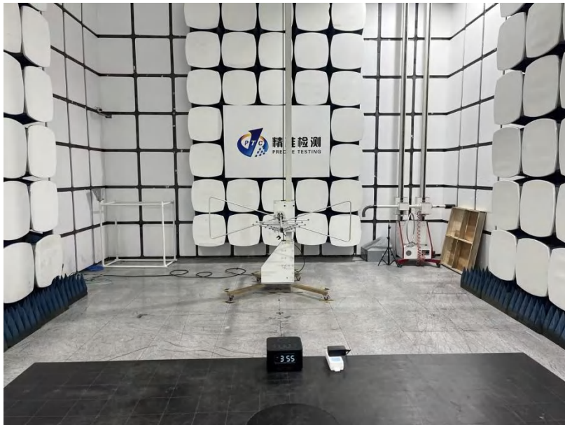
Radiated Emissions From 30M-1GHz
