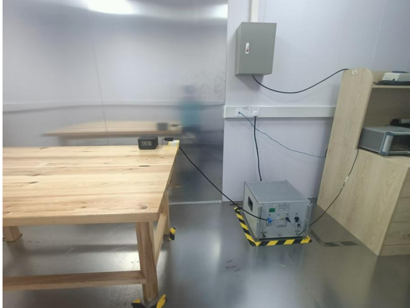
Radiated Emissions From 30M-1GHz
