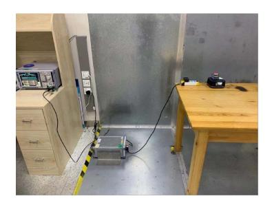
Radiated Spurious Emissions Test Frequency From 9KHz-30MHz
