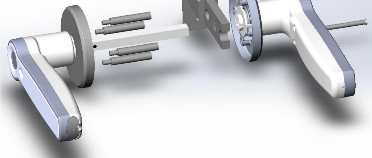
Install step 4: Install the rear panel and handle
