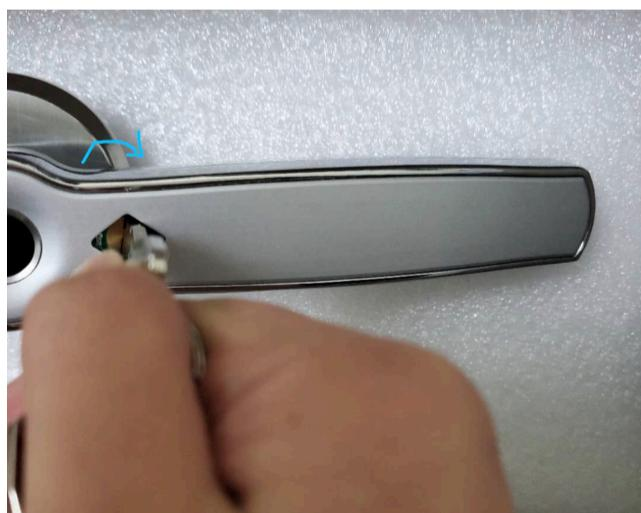
Insert the mechanical key, rotate about 15-20 degrees clockwise and hold it for about 5 seconds, (firstly, the green light will beep) until the red light is beeping, then immediately return the mechanical key back, then will see the long light-up green light is on with long "beep ~" sound. All data stored are deleted.
