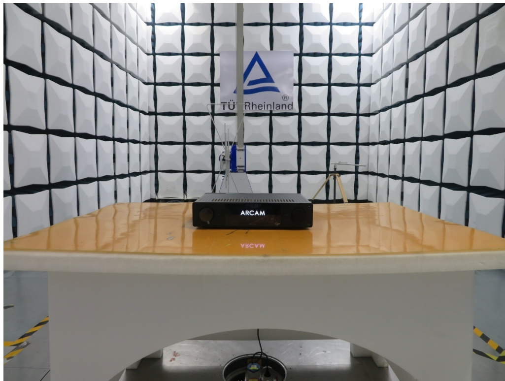
Photograph 4: Set-up for Radiated Spurious Emission, Above 1GHz
