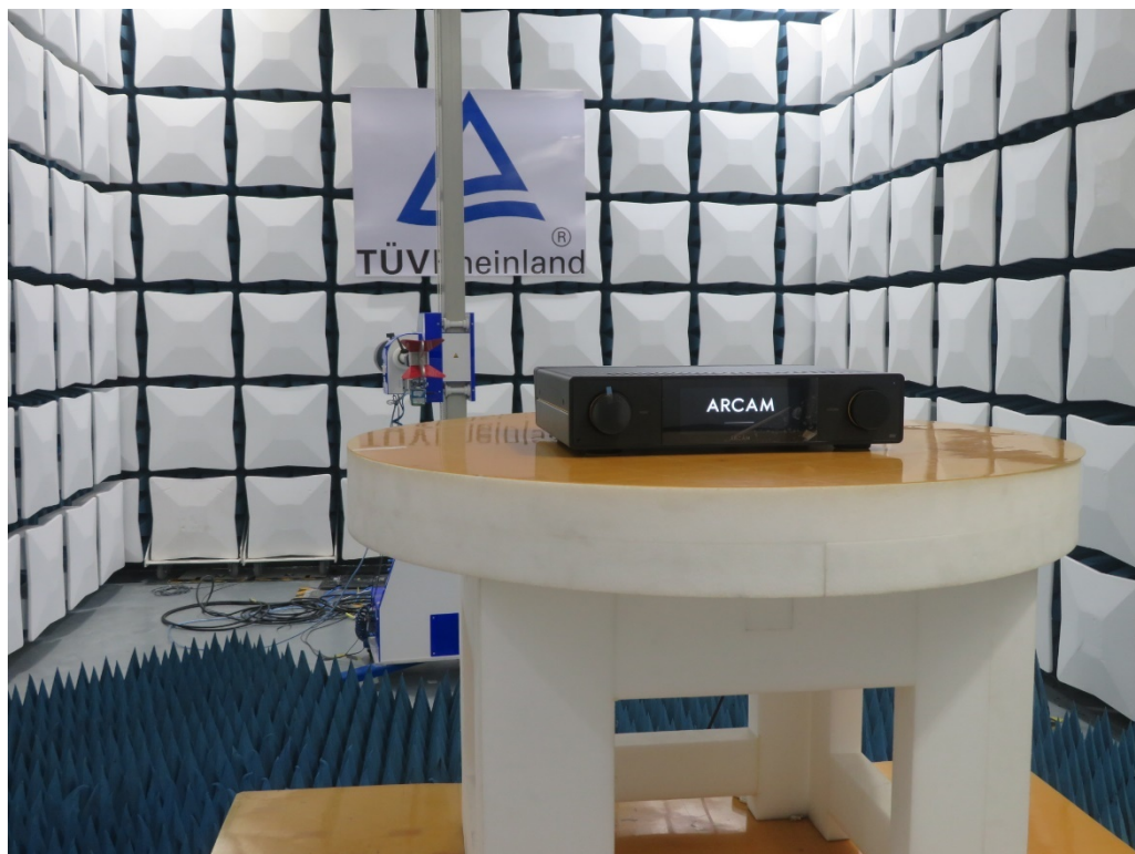
Photograph 4: Set-up for Radiated Spurious Emission, Above 1GHz
