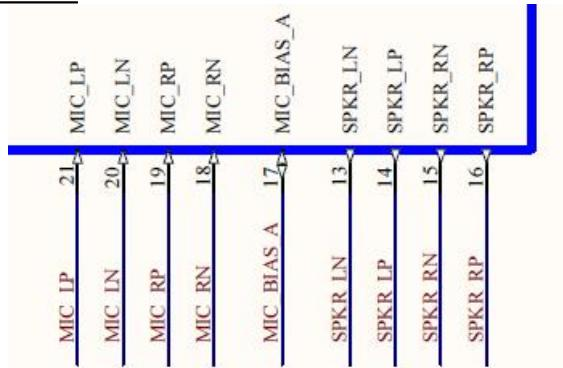
All analogue inputs are DC coupled and must be externally ac coupled for correct operation.
