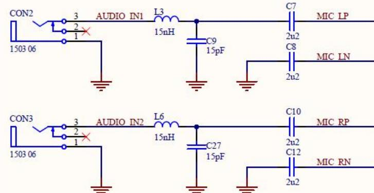
One 2-pole audio jack providing single mono audio source, unused inputs are AC grounded
