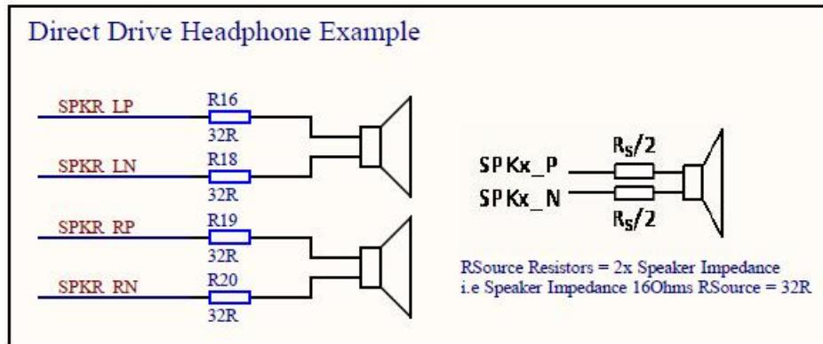
To achieve optimal audio performance in direct drive applications the DACs should operate at close to the maximum output voltage of 1Vrms. This can be achieved by adding source resistors between the output terminals and the speaker driver, the value of which are double the rated speaker impedance. i.e., for  $16\Omega$  speakers use  $32\Omega$  resistors, for  $32\Omega$  speakers use  $64\Omega$  resistors.
