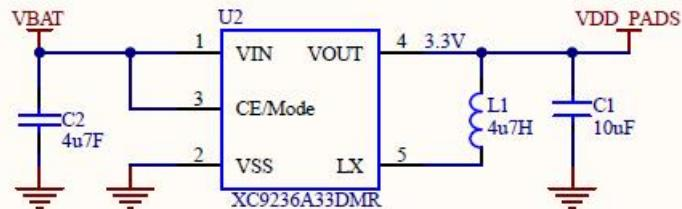
To save the cost of an external regulator the VDD\_PADS input can be connected direct to the battery input as long as all digital peripherals are tolerant of the variation of the battery voltage over its entire operating range of 2.8V to 4.24V (VFloatmax).
