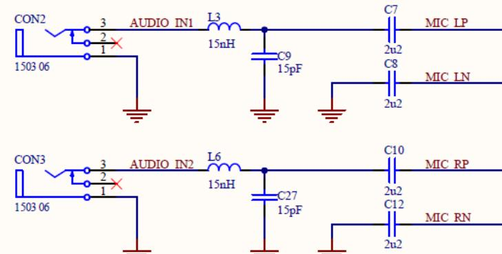
One 2-pole audio jack providing single mono audio source, unused inputs are AC grounded
