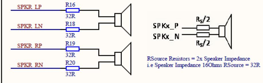
To achieve optimal audio performance in direct drive applications the DACs should operate at close to the maximum output voltage of 1Vrms. This can be achieved by adding source resistors between the output terminals and the speaker driver, the value of which are double the rated speaker impedance. i.e., for 16Ω speakers use 32Ω resistors, for 32Ω speakers use 64Ω resistors.
