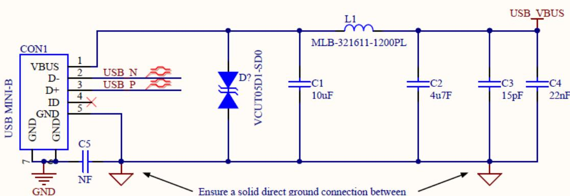
Isolate the shield ground from the board main ground. A Ferrite bead or decoupling capacitor can be added for frequency specific filtering.
