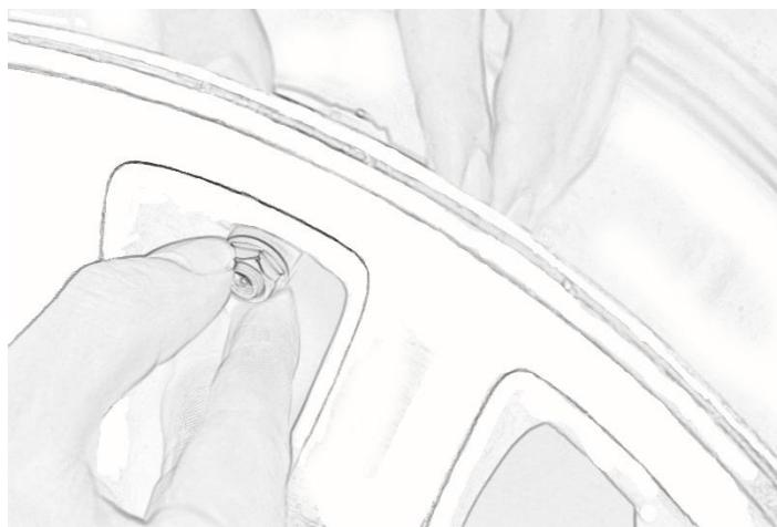
Step 2: Fix the sensor on the air nozzles with the sensor fixing screw. Note that the sensor should be close to the hub with a torque of 4N•m.
